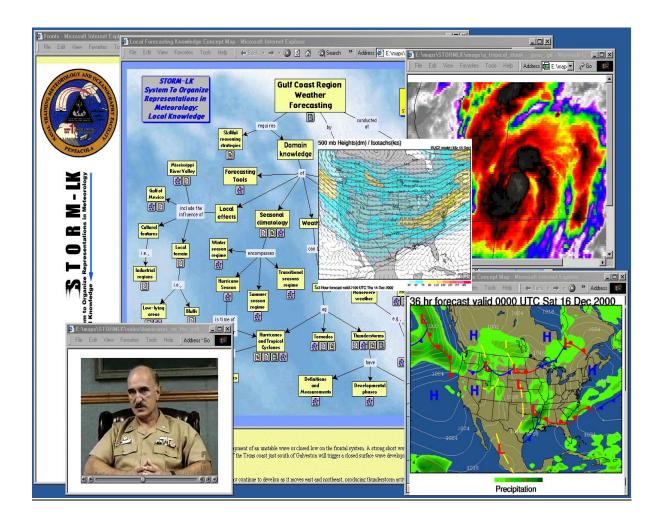
What cannot be expressed in these static Figures is that STORM-LK allows one to access all of the real-time, animated data types and data fields that are used in weather forecasting radar loops, satellite image loops, outputs of computer forecasts, prognosis charts, etc. and one can do so within the context of a set of Concept-Maps that provide the explanatory glue that makes the forecasting process hang together.
